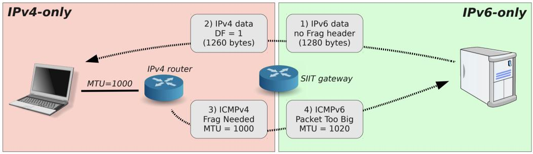
• A link in the IPv4 path towards the client may have an IPv4 MTU smaller than 1260 bytes
